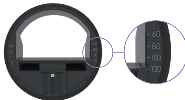
Example of an adjustment at 120 m 3 /h: regulator set at the '120' mark on the right
